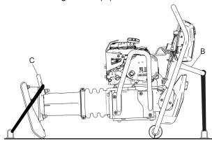
When moving short distances, the machine can be tilted forward, so that it rests on the plastic wheels on the handle. Lift with the lower lifting handle (D) and roll the machine forwards and backwards.
