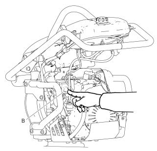
4. Close the choke (D) if the engine is cold; if the engine is warm or the ambient temperature is high, push the choke in halfway or leave open.
