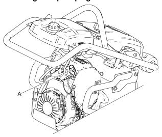
Check and clean and if necessary replace the spark plug (A).
