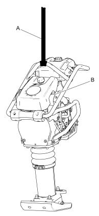
2. The lifting equipment must be in dimensioned in order to fulfil all regulations. Before lifting check that shock absorbers (B) and lifting eye (A) are correctly attached and not damaged.
