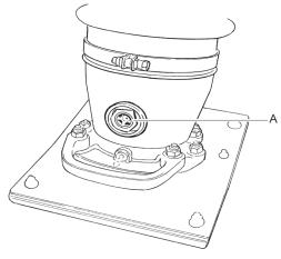
Check the oil level in the spring-loaded leg through the sight glass (A).
