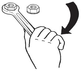
Check and if necessary tighten screws and nuts.
