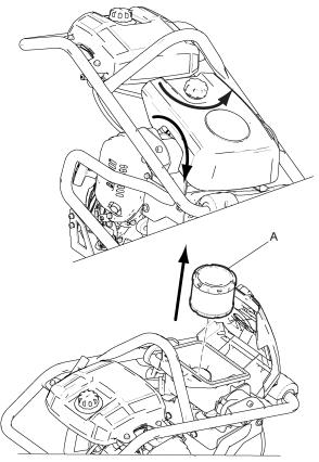
Check and clean the air filter (A).
